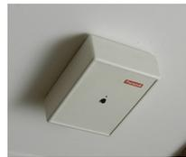
A Tunstall temperature extreme sensor monitors for low and high temperature extremes in addition to the rate of rise in temperature. This would help protect Jack from a build up of heat in the kitchen or sustained periods of cold weather.
