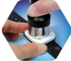
Using the battery replacement tool; turn the cover quarter of a turn clockwise to the right to close it.
