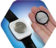
Remove the battery cover and o-ring.
