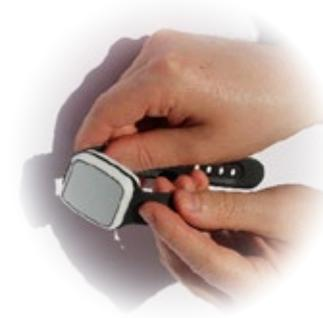
Holding onto the existing wrist strap and the Vibby gently pull until the retention features click out of place. Repeat this process for the remaining side of the strap.
