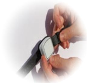
Pull the top of the wrist strap onto the Vibby. Ensuring the retention features line up with their holes and the edges fall within the enclosure.
