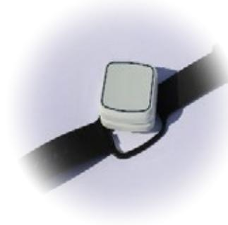
After the retention features have been removed from both sides of the Vibby; it will easily come out of the wrist strap.
