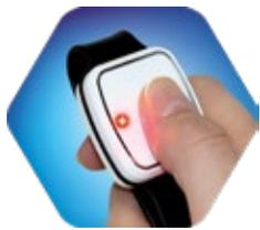
Release the button when the red LED starts flashing.
