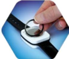
Replace the existing o-ring (D6654020A) with a new o-ring.
