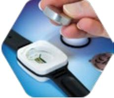
Insert the new battery with positive contact side up.
