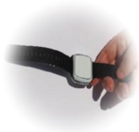
Gently pull the straps backwards to simulate the device being worn on the wrist; this will test if the retention features are correctly inserted within their holes.
