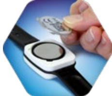
Place the cover over the o-ring and battery.
