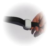
Gently pull the straps backwards to simulate the device being worn on the wrist; this will test if the retention features are correctly inserted within their holes.
