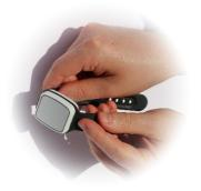
Holding onto the existing wrist strap and the Vibby gently pull until the retention features click out of place. Repeat this process for the remaining side of the strap.
